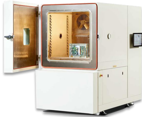
HALT / HASS (Highly Accelerated Life Test) / Highly Accelerated Stress Screen)
