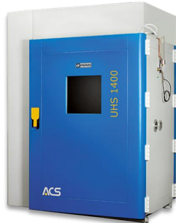
HALT / HASS (Highly Accelerated Life Test) / Highly Accelerated Stress Screen)
